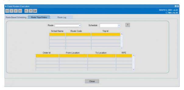
You are able to search for the information via two different filters. You can either search by "Route" or by "Schedule". The route is referring to the fixed route ID which was set up in fixed routes maintenance. The ? button activates the filter.
