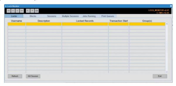
To test this on a test system Edit a Trip in the Trip Manipulation screen then Open Lock Monitor, you will see that you have particular tables locked relating to the trip you are editing. Now open two C-TMS sessions with different user ID's and use both to access the same trip in Trip Manipulation. One user will be informed that the other user has the trip locked. (Do not try this in a production environment! Make sure you are logged into a test system first.)
