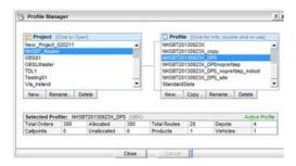
As with the PC version, DPS requires that the data parameters and optimisation configurations are set up within each profile. A profile can represent a series of successive operational days, however, each profile will be used to plan a single day or transport order demand. Each depot will be planned separately in a DPS profile.
