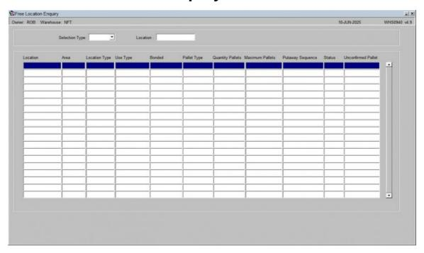
By checking within Free Location Enquiry it is possible to see key location setup data, such as how many pallets and pallet types are allowed in a location. The status of the location, (7 is full and 6 is available). And also the Putaway Sequence for each of the individual locations.
